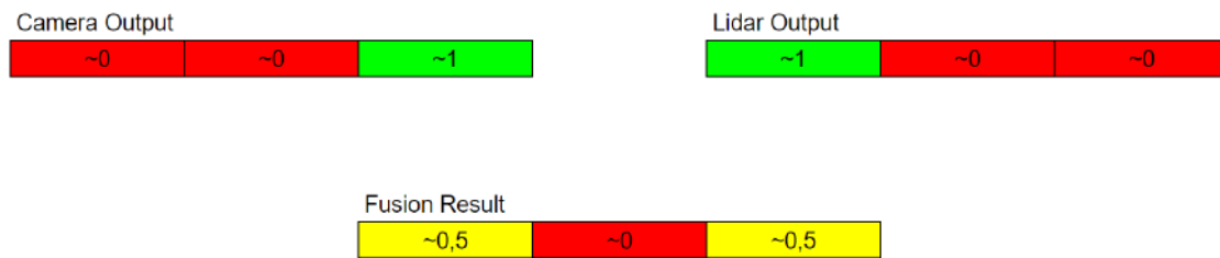
Figure 4.5: Illustration of a Naive Fusion Method
