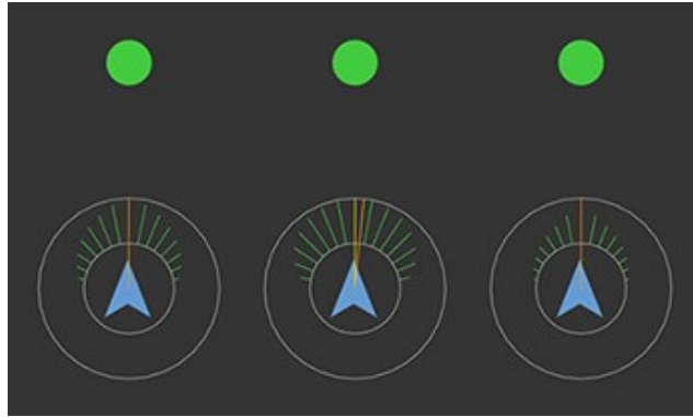
Figure 3.4.: The effects of different mapping types for value mapping. From left to right: inverse linear, inverse quadratic, inverse square root.
